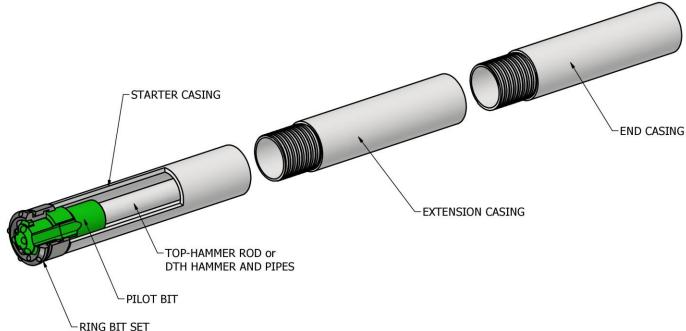
On top of the tunnel applications, Model T is also suitable for many other casing drilling works like small anchor drilling, micro piling and drainage holes. Everyplace where small diameter casings are used.
